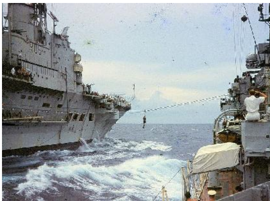
A good picture of a jackstay transfer between Centaur and the Destroyer Solebay taken in 1961 whilst the ships were on passage Ceylon to Aden.
